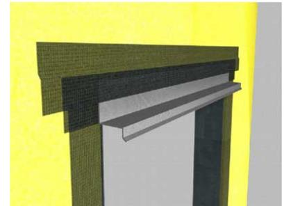
Overlap AquaFlash System over flashing leg minimum 2 in (51 mm)
